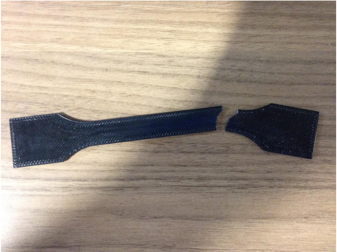
Figure 15: The failed test sample
