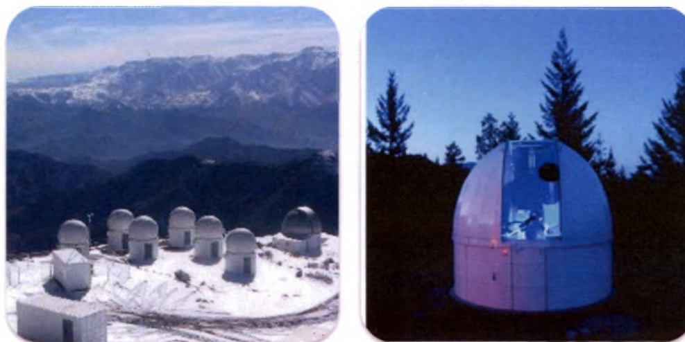
Figure 3: Robotic telescopes. [Left] Panchromatic Robotic Optical Monitoring and Polarimetry Telescopes (PROMPT) is an array of six 0.41-meter telescopes located in CTIO in Chile. [Right] The Gamma-ray Optical Robotic Telescope (GORT) is a 14" diameter telescope located near Santa Rosa, California.
