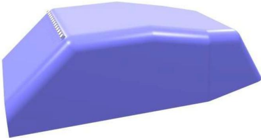
Figure 1.4 Blunt body with VGs placed behind shoulder of boat-tail.
