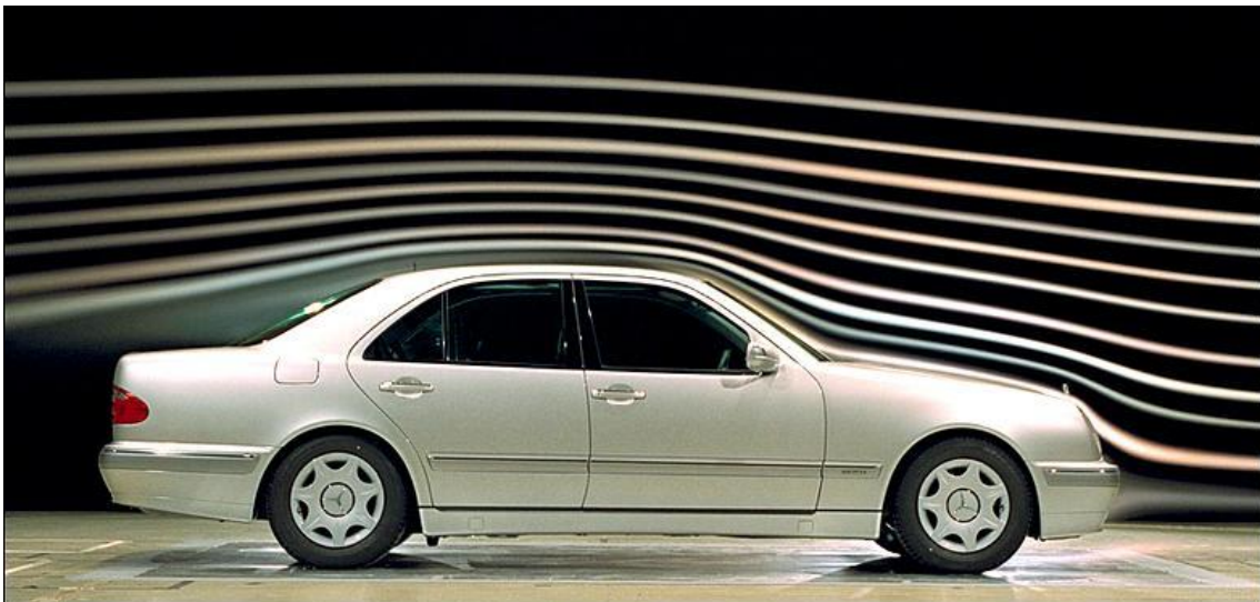
Figure 2.3 Streamlines around a stationary vehicle [14].
