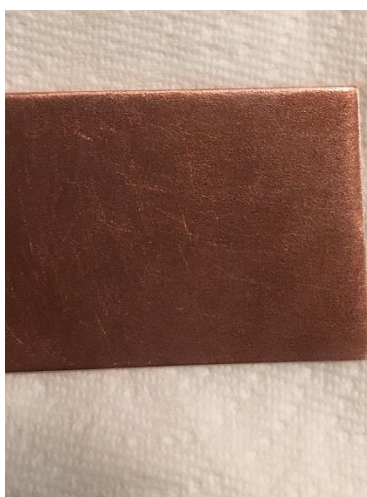
Figure 7.1 Copper sample after copper strip test showing slight tarnish
