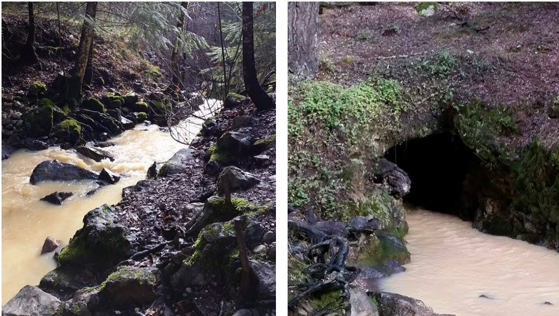
Figure 28. Sample Day Five, 2/8/2015, Hiller Tunnel Effluent During Storm Event. High turbidity and discharge (left) and flow downstream to Humbug Creek (right).
