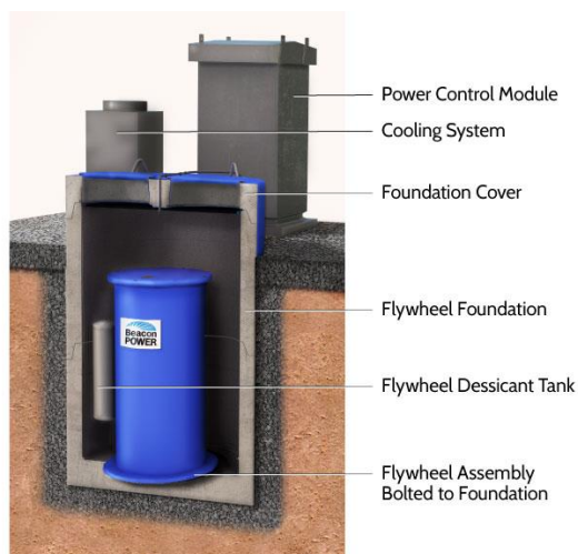
Figure 18. Beacon Power System Installation
